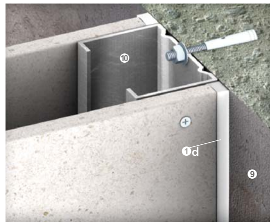
Control joint seals in junctions between a lightweight partition and a concrete or masonry wall
